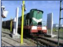
Rail Monitors at Batumi Seaport
